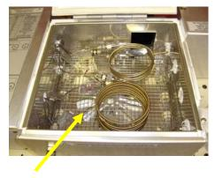
Two 2 meter long packed columns are installed in the GC's column oven, a Silica Gel column and a Molecular Sieve 13X column. The two columns separate the transformer gases in the same way that SRI's Multiple Gas#1 GC configuration does. To understand how the two columns work to perform the separation is would be useful to review the Multiple Gas#1 GC instructions ( download from www.srigc.com ).
